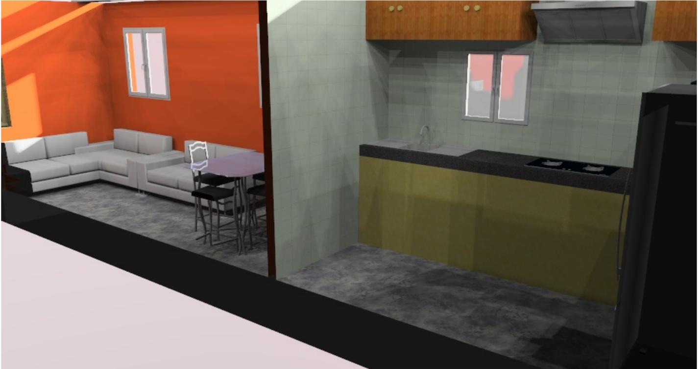
Interior elevations are very similar to exterior elevations in purpose. With interior elevations, you can create a view with just the baseboard, windows, and crown molding or a room with all of the furnishings. Elevations are extremely useful when constructing a room such as a kitchen or a bathroom, which require visualization of built-in elements.
